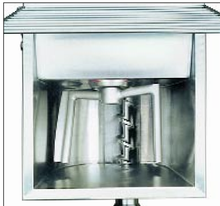
Mixer with forward and reverse automatic for blending and as automatic feeder
