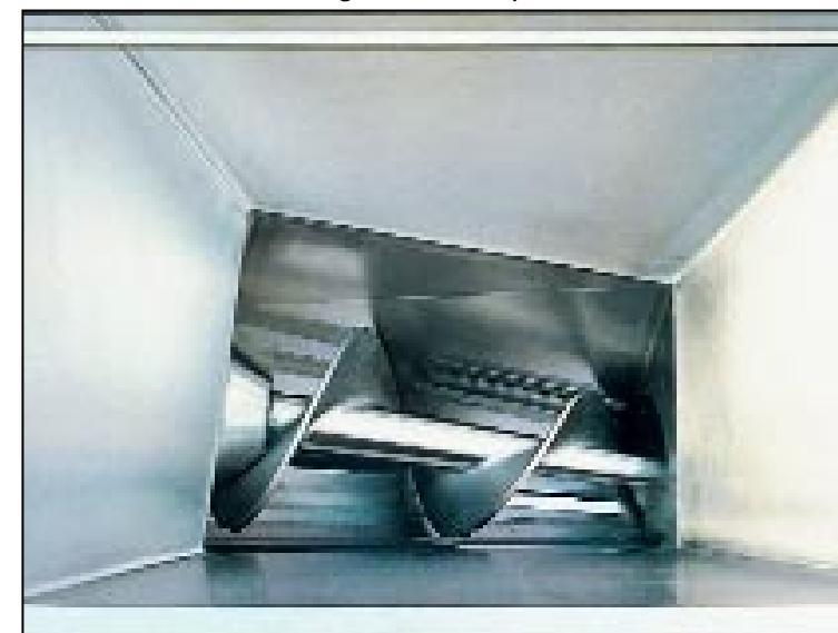
wide conical feeding worm of up to 270 mm diameter
